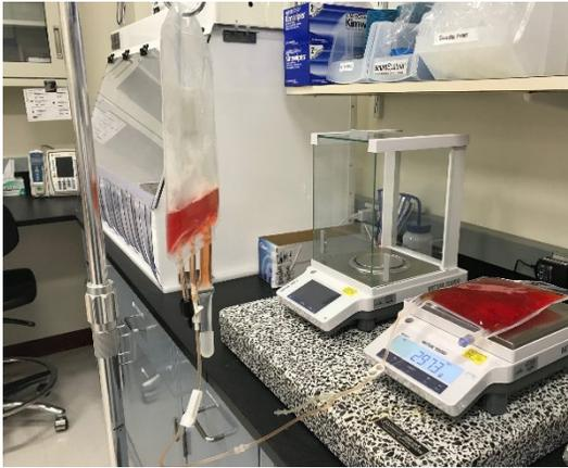
Figure 2. Addition of culture media from media bag to VueLife® culture bag. Bag contents can be transferred via gravity and volume can be tracked by using a lab scale.
